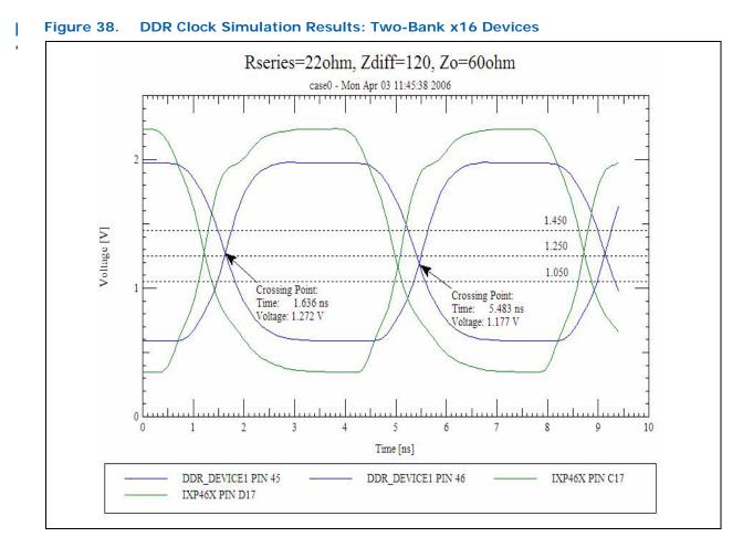
The differential-clock-circuit simulation in Figure 38 shows that the voltage waveform meets the DDR device input voltage requirements. The crossing point for the clock input must occur between  $V_{ix(min)} = 1.05$  V and  $V_{ix(max)} = 1.45$  V and have a minimum peak to peak swing of 700 mV. The receiver input waveform must also not exceed a maximum voltage of  $V_{in(max)} = 2.8$  V or the minimum voltage of  $V_{in(min)} = -0.3$  V.
